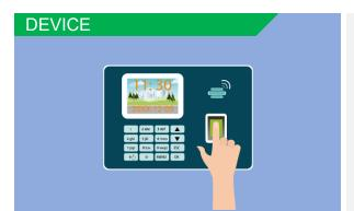
As the name indicates it is used to configure the time and attendance terminals with options such as authentication mode, attendance mode, communication details etc. It is also used to transfer finger print templates and to download the transactions.
